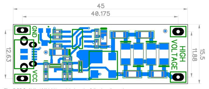
The DCDC\_3V3\_400V\_V1 module has the following dimensions:
