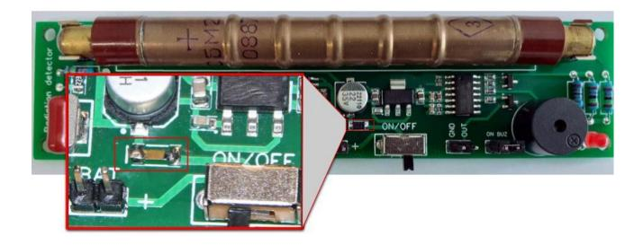
Fig. GGreg20\_V3 Reverse Polarity Protection Diode Manual Replacement Example
